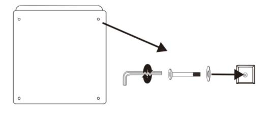
STEP 2: Unfold connection clips to poke out from bottom of the item and then place in slideway parts at bottom of another item
